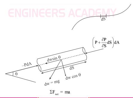
$$pdA - \left(p + \frac{\partial p}{\partial s}ds\right)dA - \rho g\partial A\partial s\sin\theta \ = \ ma$$
