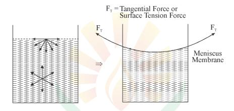
It is defined as a tangential force acting on a per unit length of free surface of liquid Formula
